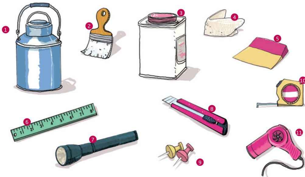
1 Primer (PM02, PM04) 2 Brush 3 Cleaning solvent (alcohol, white gasoline or lacquer thinner) 4 Lint 5 Plastic applicator 6 Steel ruler 7 Torch 8 Stanley knife (45° angle) 9 Needle or pin 10 Measuring tape 11 Hair dryer 12 Other : sandpaper, putty stick, sealer, masking tape, gloves
